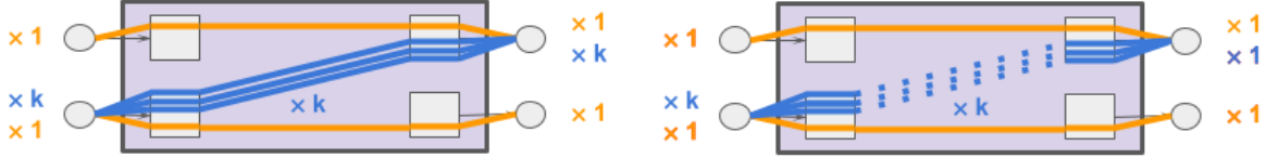
(a) In the maximum throughput allocation, both orange flows have rate 1, and all blue flows have rate 0, leading to throughput 2. (b) In the max-min fair allocation, all flows have rate 1/(k+1) , leading to throughput 1 + 1/(k+1) , which approaches 1 as k grows large.
